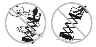
Do not drive the machine on or near uneven terrain, unstable surfaces or other hazardous conditions with the platform raised.
